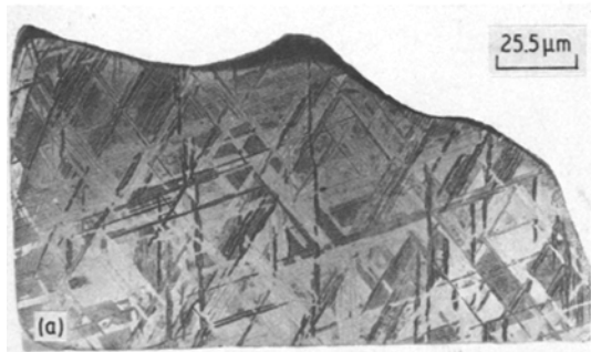
Figure 9 (a) Survey of Gibson meteorite showing exclusively Widmannstätten kamacite ( \alpha -Fe) (cf. Fig. 3); Etching agent 3. (b) \alpha - \alpha and \alpha - \gamma cracks which must have formed at low temperature T_2 . There is no evidence for T_1 cracking in the investigated part of this meteorite; unetched.
